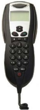
The handset is compact and includes an inbuilt ring alert as well as providing for private conversations in place of hands-free mode.
